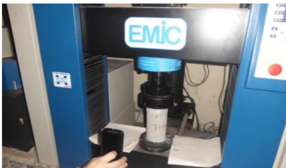
Fig. 6 Equipment for testing compression
