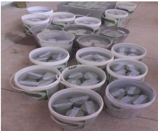
Fig. 5 Specimens immersed in water.
