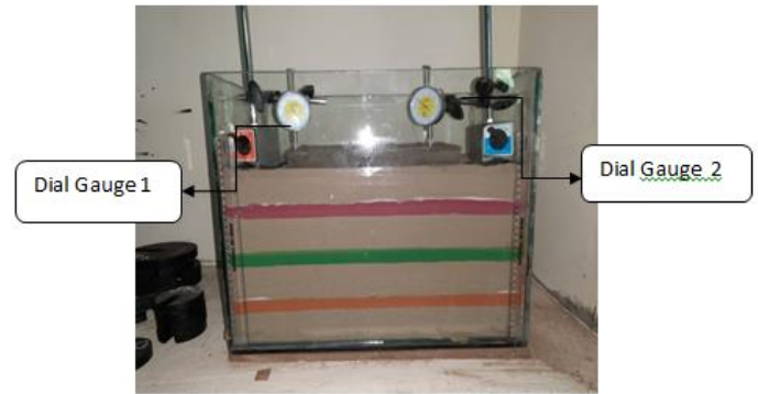
Fig 2. Dial Gauges Used for Settlement
