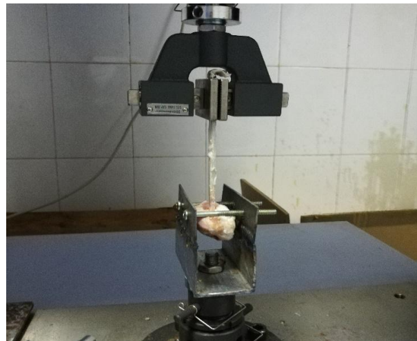
Fig 3. The specimen in the material testing machine (MTS). The patella is fixed to the base of MTS, the free ends of the graft are fixed to the upper loop of MTS.
