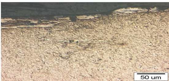
Fig. 3 Cross section of Race 1 with higher hardness of surface, after durability test. The white fields represent plastically deformed martensite and/or rests of fretting corrosion on the loaded area.
