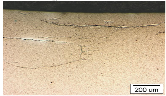
Fig. 4 Cross section with cracks below the softer surface of Race 2, after durability test. Contact fatigue cracks propagating parallel to the loaded area.
