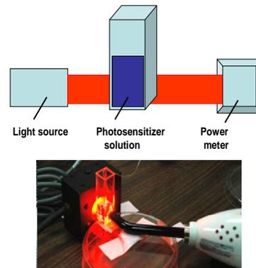
Fig. 1 Experimental setup shows an incident red light and the transmitted light intensity ( $I$ ) measured by a power meter,
