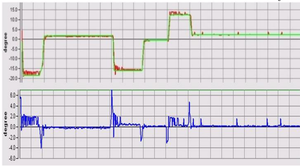
Fig. 12 Comparison between estimation of orientation and the actual orientation using GUI. Green: reference signal (set point), red: the result of estimation filter, blue: the difference between the estimation and the actual orientation.
