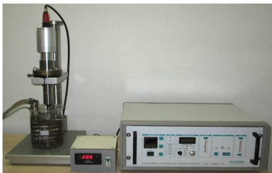
Fig. 1 Cavitation stand composed of vibrator apparatus, ultrasound generator and digital thermometer
