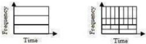
Fig. 1 Standard FFT (on the left) and MR FFT (on the right)
