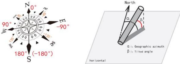
Fig.9 Geographic Azimuth and the Tilted Angle
