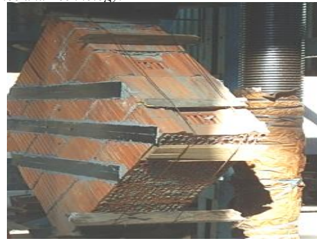
Image 1 Marking the position of the lamellas
