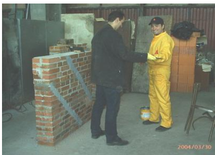
Image 1 Marking the position of the lamellas
