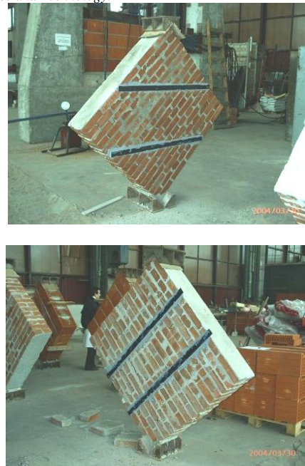
Image 2 Sample made out of solid bricks prepared for reinforcement
