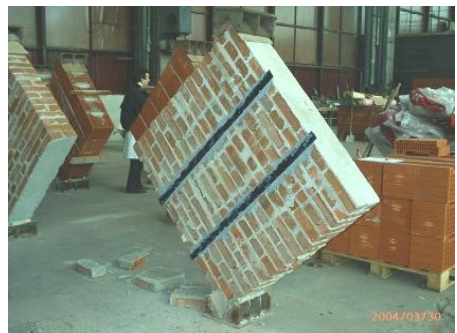
Image 2 Sample made out of solid bricks prepared for reinforcement
