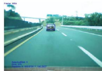
Fig. 12 Obstacle Detection. The corresponding object identified as an obstacle is easily tracked through time with a blue frame in the RGB space.
