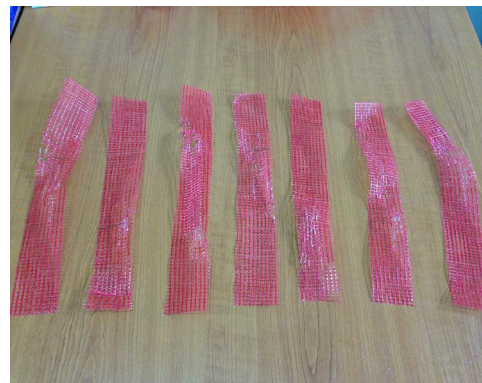
Picture 2. Specimens after determining the tensile strength
