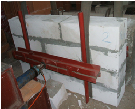
Picture 5. Specimen for testing in flexure perpendicular to the plane of the wall and perpendicular to the laying joints
