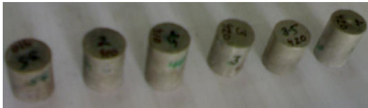
Figure 4: Sintered billets of aluminium powder
