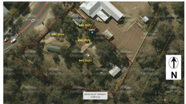
Figure 6: Location of Lot 22 (66) Royal Street, Kenwick WA City of Gosnells, South East Metropolitan Tests Locations: Bore Hole (BH), Dynamic Cone Penetration (DCP) and Field Permeability Test (FPT)
