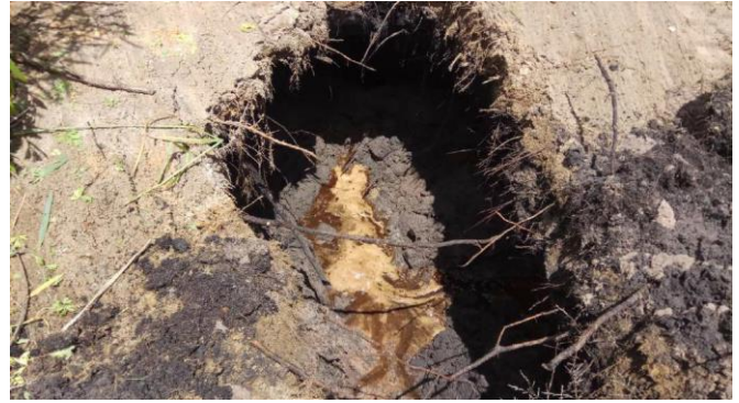
Figure 17: Soil Profile, Test Pit location (TP5) and ground watertable encountered at a depth of 0.9 m
