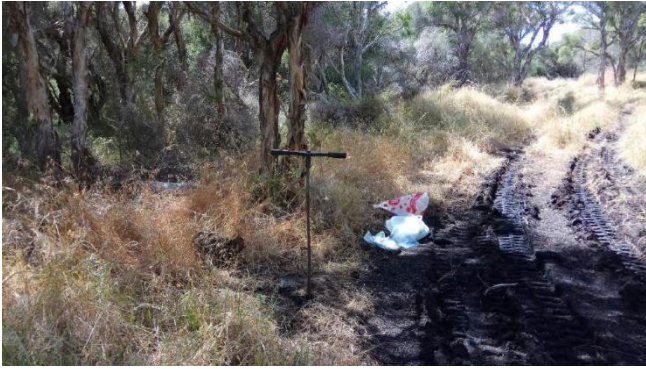
Figure 53: Photo 16. Subsurface probing and Acid Sulphate Soil (ASS) sampling at Bore Hole location (BH1)
