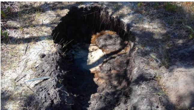
Figure 46: Photo 09: Soil collapsing into Test Pit location (TP9) & ground watertable encountered at 0.65 m depth
