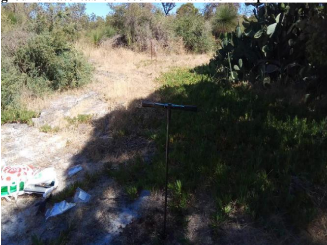
Figure 32: Subsurface Probing by Hand Auger at Bore Hole Location (BH2)
