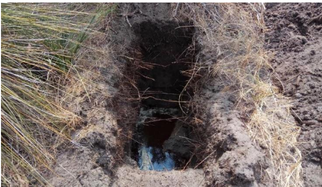
Figure 54: Soil Profile, Test Pit location (TP7) and ground watertable encountered at a depth of 1.2 m
