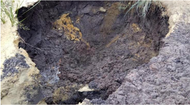
Figure 13: Soil Profile, Test Pit location (TP3) and ground watertable encountered at a depth of 1.2 m
