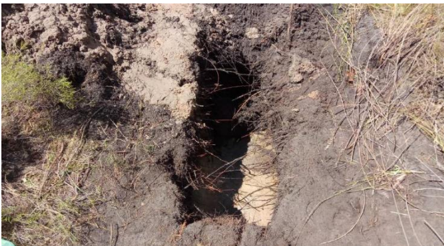
Figure 23: Soil Profile, Test Pit location (TP8) and ground watertable encountered at a depth of 0.8 m
