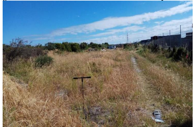
Figure 34: Subsurface Probing by Hand Auger at Bore Hole Location (BH3)
