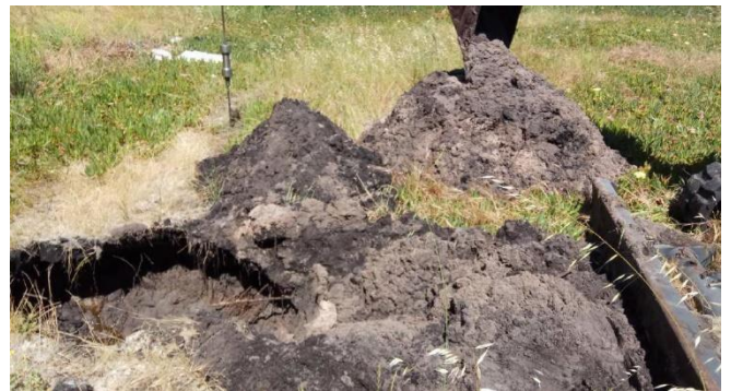
Figure 27: Soil from Test Pit location (TP10)
