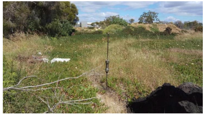
Figure 49: Photo 12: Conducted a Dynamic Cone Penetrometer (DCP) Test at Location DCP10
