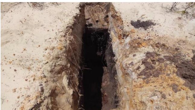
Figure 15: Soil Profile, Test Pit location (TP4) and ground watertable encountered at a depth of 2.0 m
