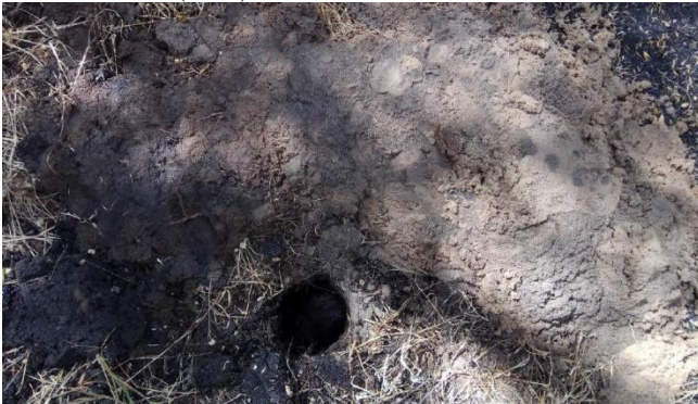
Figure 31: Soil from Bore Hole Location (BH1) and ground watertable encountered at 0.33 m depth
