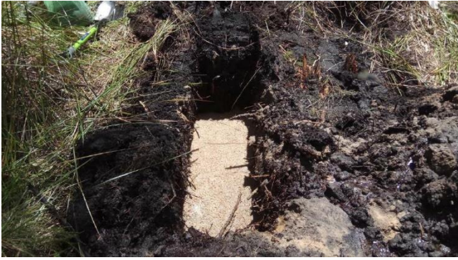
Figure 21: Soil Profile, Test Pit location (TP7) and ground watertable encountered at a depth of 0.9 m
