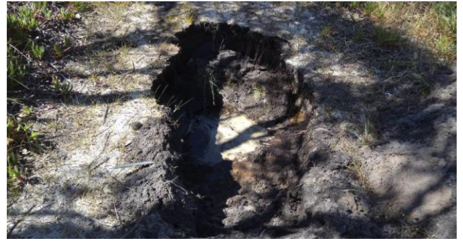
Figure 25: Soil Profile, Test Pit location (TP9) and ground watertable encountered at a depth of 0.65 m
