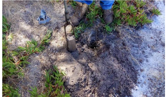
Figure 33: Soil from Bore Hole Location (BH2) and ground watertable was encountered at 0.8 m depth
