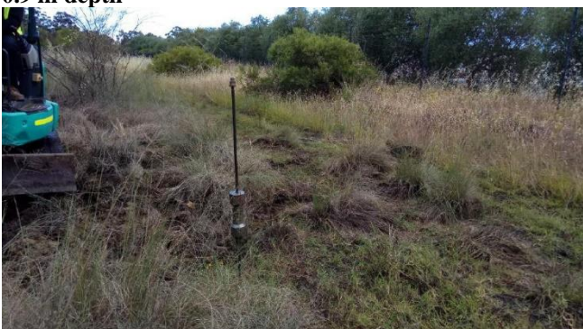
Figure 48: Photo 11: Conducted Dynamic Cone Penetrometer (DCP) Test at Location DCP6
