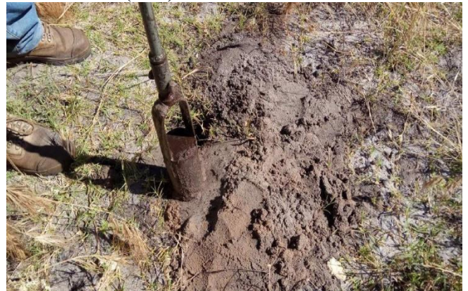
Figure 35: Soil from Bore Hole Location (BH3) and ground watertable encountered at 1.0 m depth
