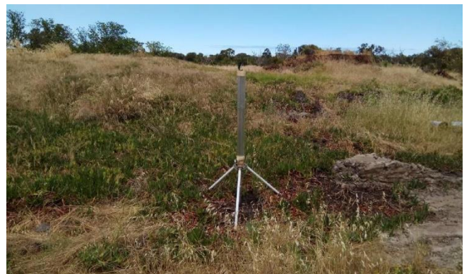
Figure 52: Photo 15: Conducting Field Infiltration Test at Location FPT4
