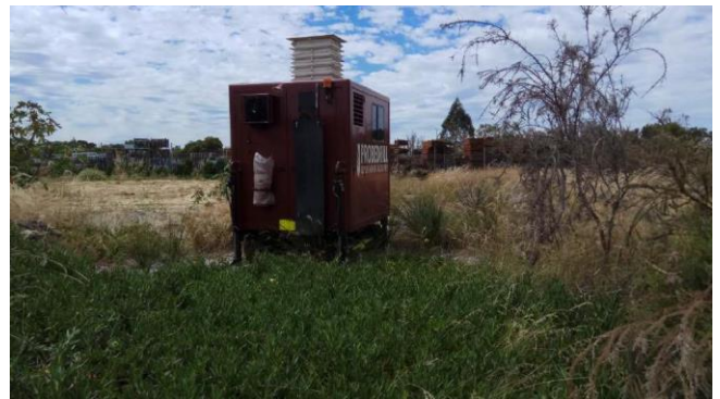
Figure 51: Photo 14. Conducting Cone Penetration Test at the location (CPT2)
