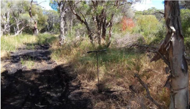
Figure 30: Subsurface Probing by Hand Auger at Bore Hole Location (BH1)
