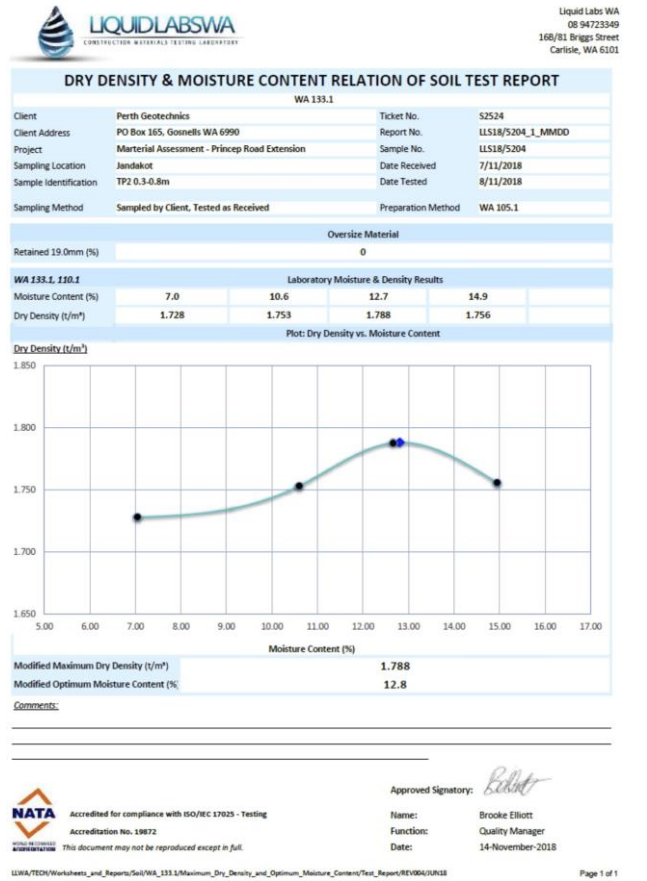
Figure 110: Max dry density and moisture content at TP2
