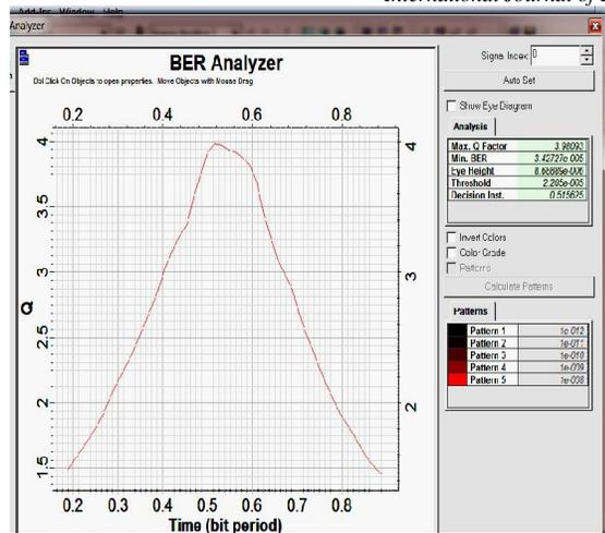
Figure 14. Received Optical Signal of Fiber length 130 km after using FBG
