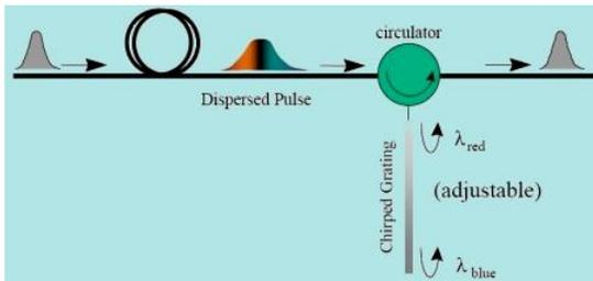
Figure 6 Chromatic Dispersion Compensation using FBD and Circular [11-13].
