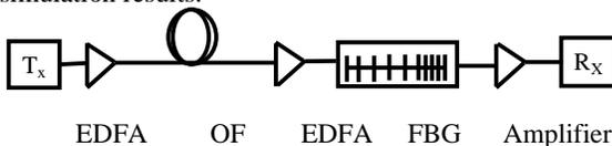
Figure6. Fiber-optic Transmission link System Block Diagram
